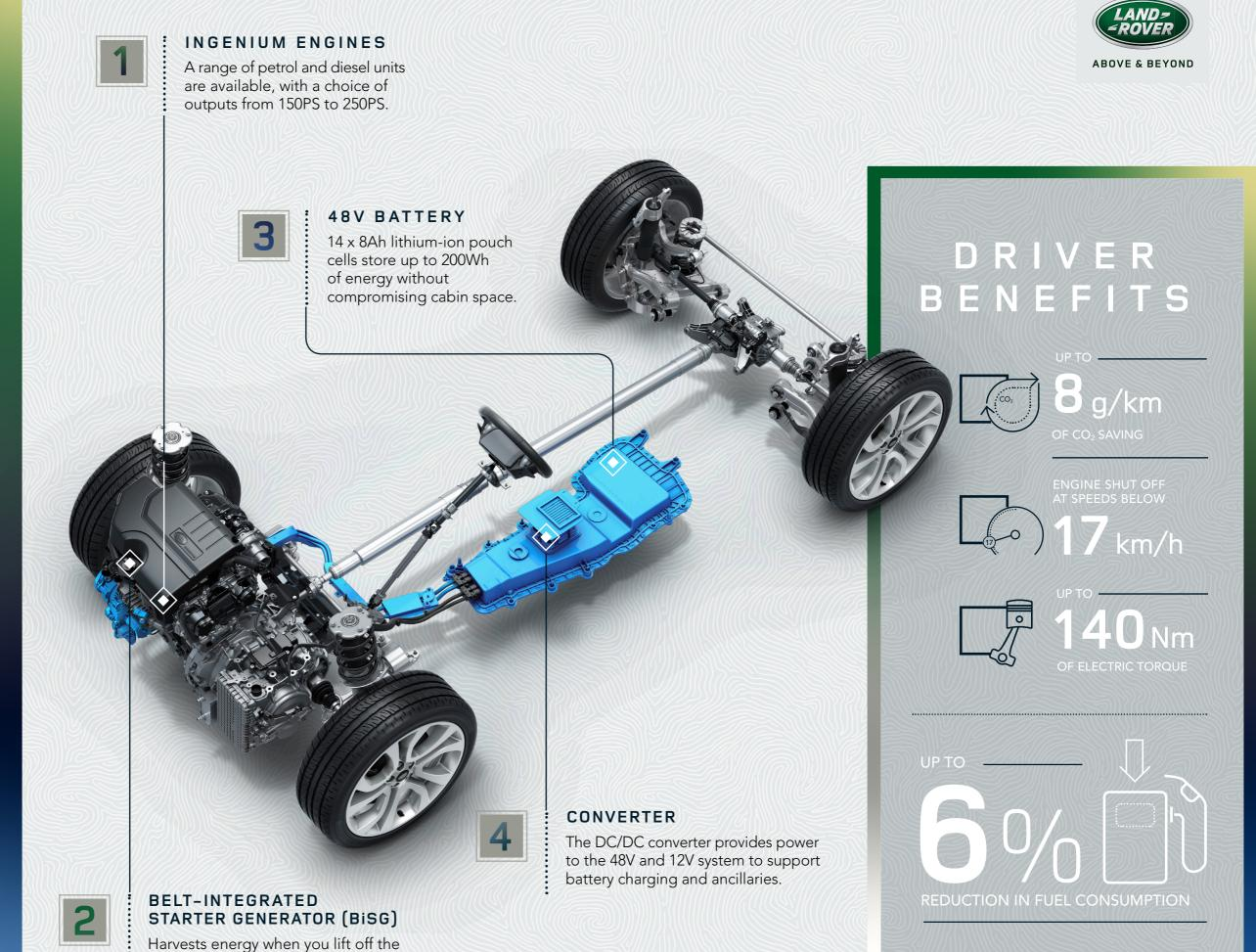
accelerator sending electricity to the battery, then redeploying it as torque to aid transient acceleration.
