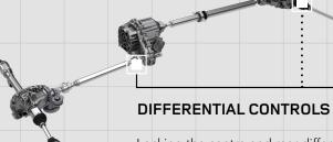
Locking the centre and rear differentials ensures peerless capability no matter the surface, as well as allowing cross-axle slip ensuring a dynamic experience on-road
