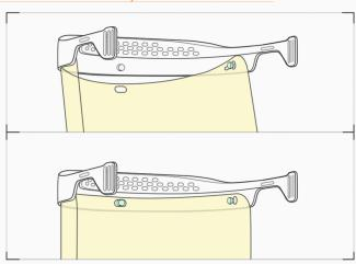
Holding the headpiece so the pins are easily accessible, gently bend the pre-cut clear plastic screen before letting go of the screen so the pins slide into their engaged position. Slowly rotate and position the screen, so that the centre peg on the headpiece protrudes through the centre slot on the screen.
