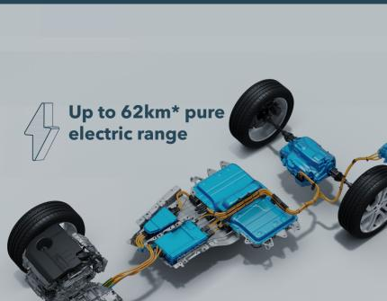
**RANGE ROVER EVOQUE PHEV P300e AWD AUTOMATIC** 1.5-litre three-cylinder Ingenium Petrol
